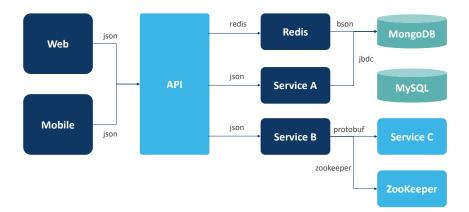
The Microservice architecture pattern corresponds to the Y-axis scaling of the <u>Scale Cube</u> model of scalability.
